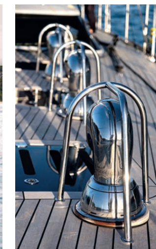
Above: stainless steel frames around the six large dorade vents increase security on the foredeck.
