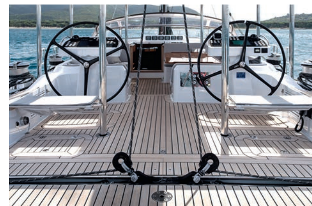
A working cockpit for the crew would normally be abaft the guests' cockpit, moving the wheels further aft
