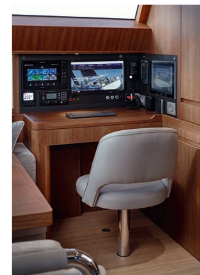
Above: nav area includes touch-screen displays for full management of the boat's systems. Above right: ladders drop down from the deckhead in every cabin
