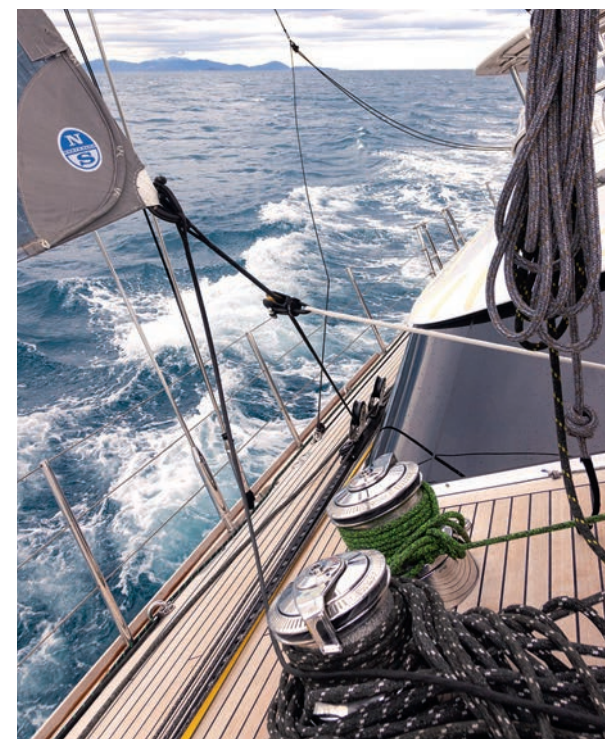
Barber-hauling the staysail significantly improved upwind performance. Extra blocks and lines together with plenty of winches allow almost any sheet or halyard to be led to any winch
